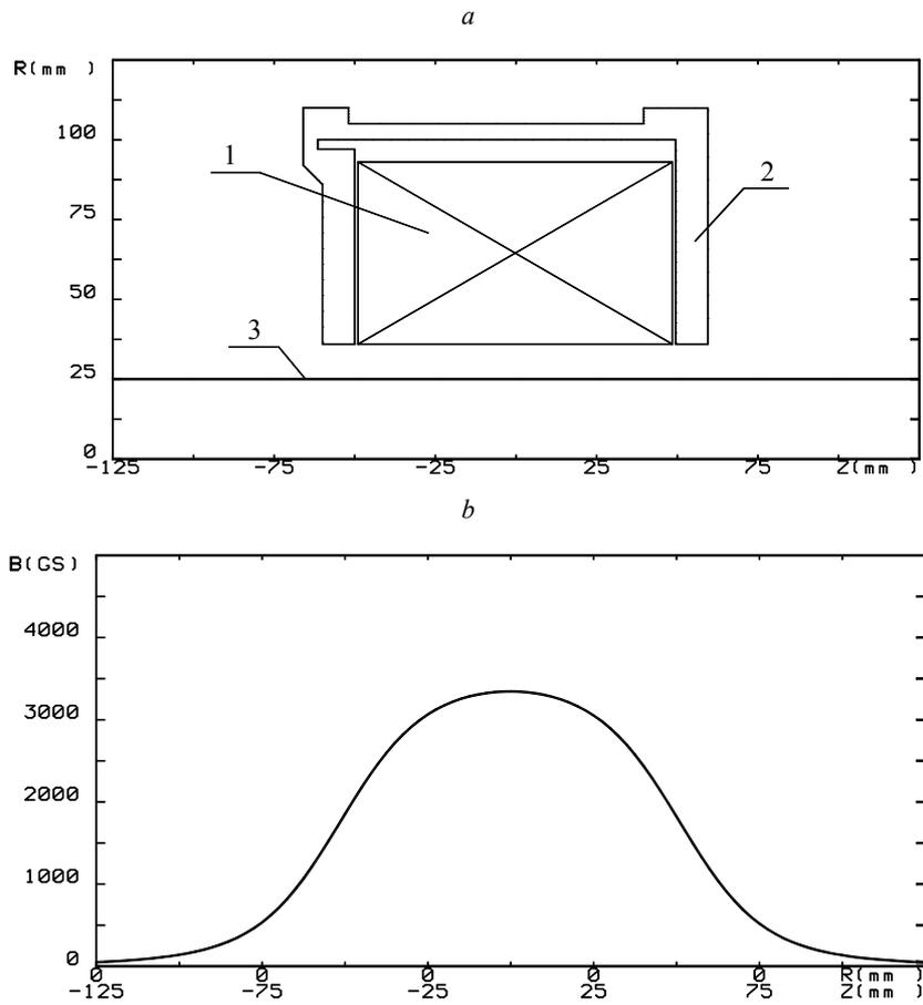
Fig. 9. Calculated geometry of the magnetic lens (a) and longitudinal distribution of magnetic field for maximum current 29,25 kA·turns in the lens winding (b). The numbers mark: 1 – current coil, 2 – magnetic field, 3 – contour of the drift tube.
