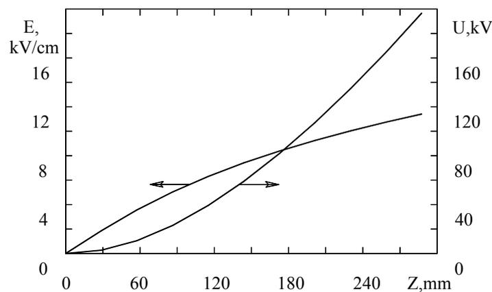
Fig. 5. Analytic distribution of the potential and the field, which provides acceleration of the negative hydrogen ion beam with initial energy of 25 keV and current of 10 mA with a constant diameter of 10 mm.
