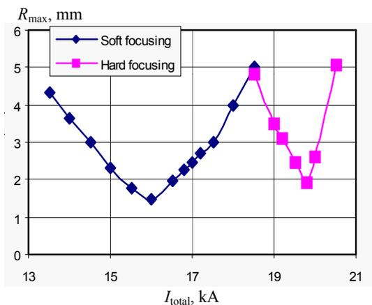
Fig. 14. Calculated dependence of maximum radius of the envelope of 95% of the H beam’s current in the charge-exchange tube on the full current in the second magnetic lens for the schemes with “weak” and ”strong” beam focusing.
