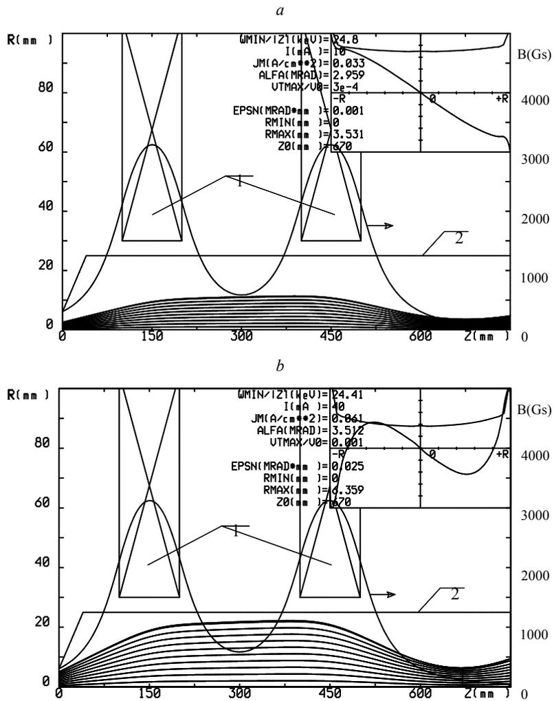
Fig. 3. Results of calculations of the transportation of 25 keV H<sup>-</sup> beam with current of 10 mA (a) and 40 mA (b) using two magnetic lenses: 1 – current coils, 2 – contour of the drift tube. On the insert in the top right corner, there are the radial distribution of the current density and the phase-plane portrait of the beam in the focal point of the second lens.
