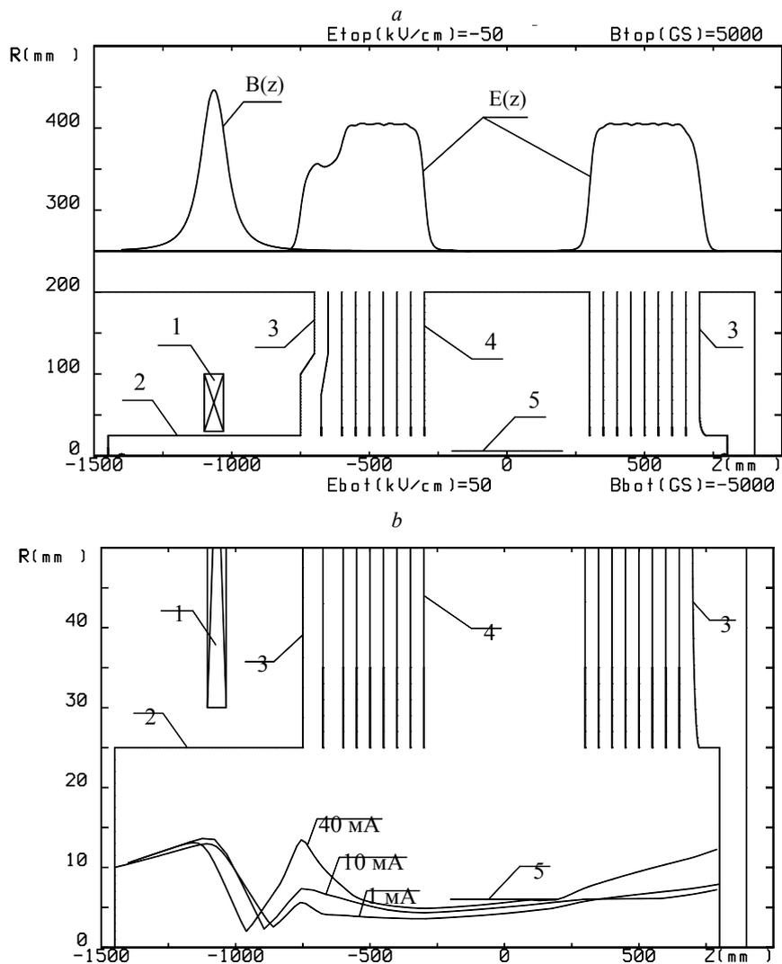
Fig. 4. Coordinated transport of 25 keV H beam in the tandem accelerator according to "strong" focusing scheme: the ion-optical path geometry, calculated longitudinal field distributions (a) and the envelopes of ion beams with current of 1 mA, 10 mA and 40 mA (b). The numbers mark: 1 - current coil, 2 - drift tube, 3 - vacuum tank, 4 - high-voltage electrode, 5 - stripping tube.
