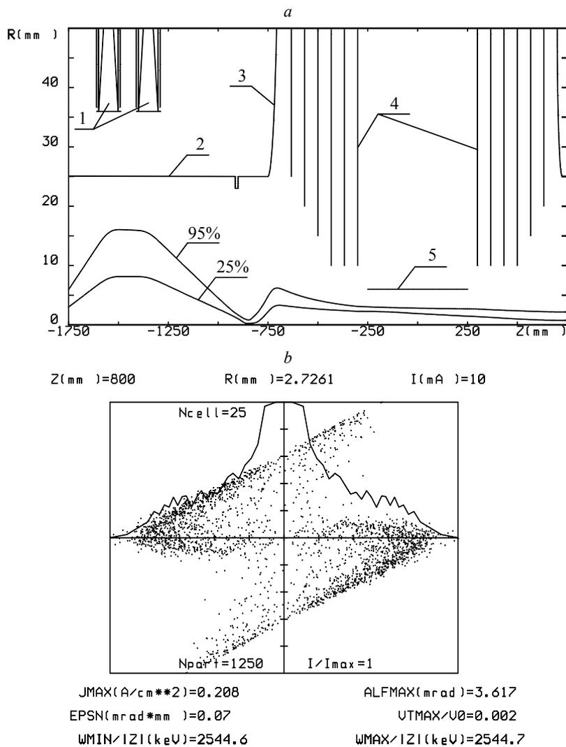
Fig. 13. Results of calculation of the ion-optical path of tandem accelerator for a scheme with "weak" focusing of a H beam with current of 10 mA and initial energy of 25 keV: *a* – envelopes of 25% and 95% of the beam's current; *b* – radial current density distribution and beam emittance at the outlet from the accelerator. The numbers mark: 1 – magnetic lenses, 2 – drift tube, 3 – vacuum tank, 4 – high-voltage electrode, 5 – charge-exchange tube.
