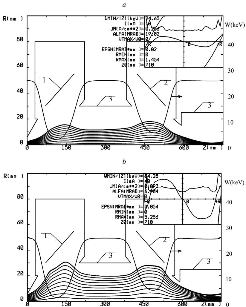
Fig.2. Results of calculations of the transportation the 25 keV H beam with a current of 10 mA (a) and 40 mA (b) using two electrostatic lenses: 1 – the first decelerating electrode, 2 – the second decelerating electrode, 3 – contour of the drift tube. On the insert in the top right corner there are the radial distribution of the current density and the phase-plane portrait of the beam in the focal point of the second lens.
