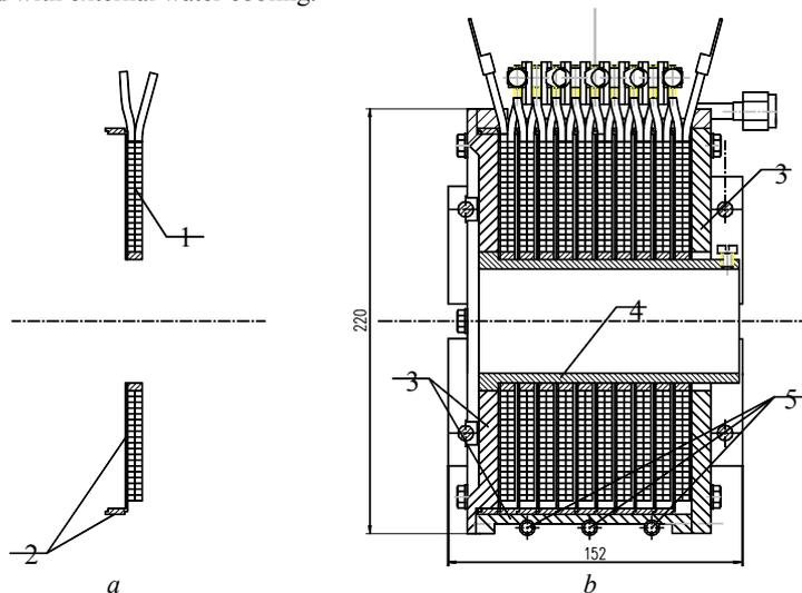
Fig. 8. Magnetic lens draft: base winding module (a) and a ready-assembled magnetic lens (b). The numbers mark: 1 – a current bus-bar, 2 – aluminum disc, 3 – magnetic shield, 4 – lens frame (stainless steel), 5 – pipes of cooling system.
