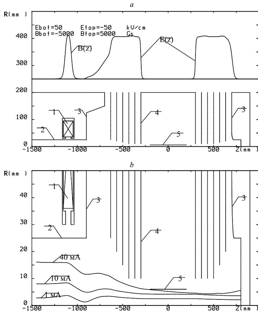
Fig. 7. Coordinated transport of 25 keV H beam through tandem accelerator according to simplified "weak" focusing scheme: the ion-optical path geometry, calculation longitudinal distributions of the field (a) and the envelopes of ion beams with current of 1 mA, 10 mA and 40 mA, spanning 95% of the current (b). The numbers mark: 1 – the magnetic lens, 2 – drift tube, 3 – vacuum tank, 4 – high-voltage electrode, 5 – charge-exchange tube.
