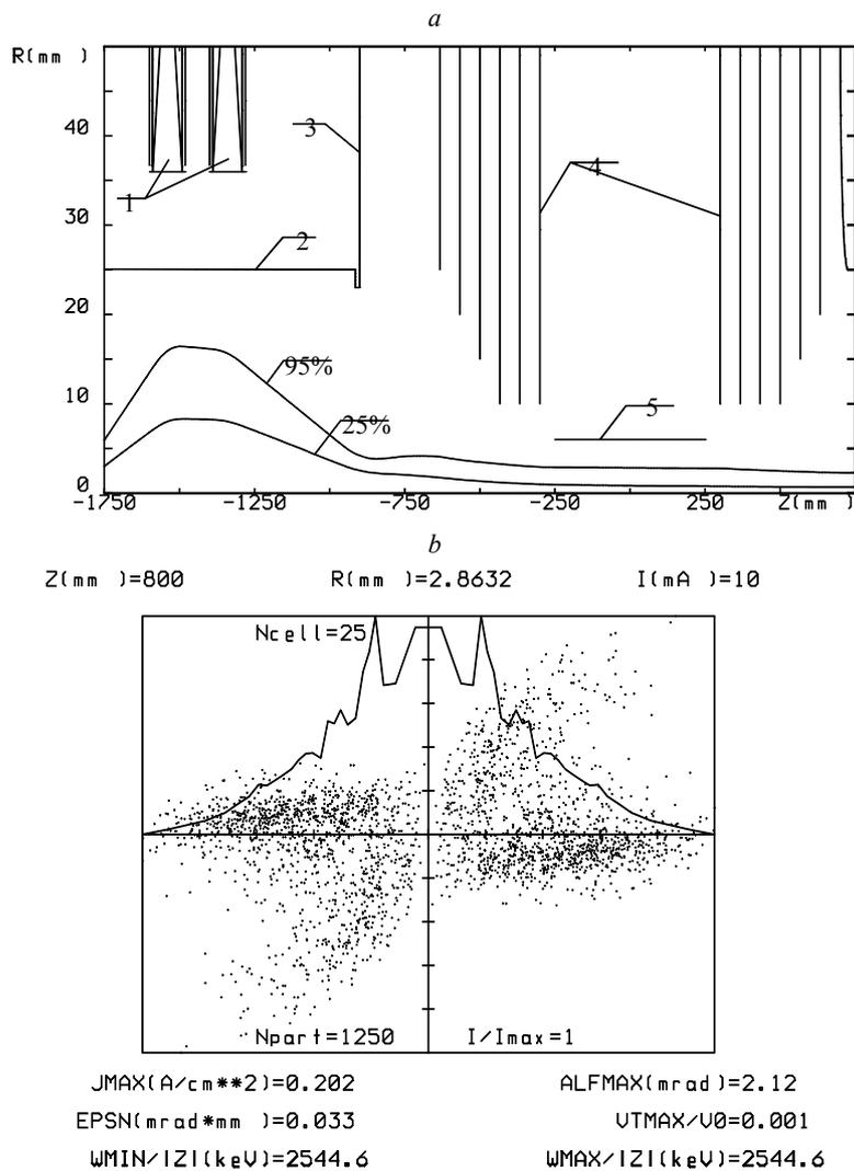
Fig. 11. Results of calculation of the ion-optical channel of tandem accelerator for a scheme with “weak” focusing of  $H$  beam with current of 10 mA and initial energy of 25 keV: *a* – envelopes of 25% and 95% of the beam current; *b* – radial current density distribution and beam emittance at the outlet from the accelerator. The numbers mark: 1 – magnetic lenses, 2 – drift tube, 3 – vacuum tank, 4 – high-voltage electrode, 5 – charge-exchange tube.
