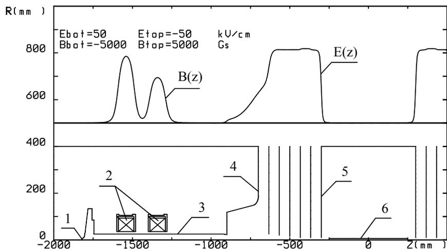
Fig. 10. Geometry of the ion-optical channel of a tandem accelerator and calculation longitudinal distribution of the field for the scheme with “weak” focusing of a  $H$  beam with current of 10 mA and initial energy of 25 keV. The numbers mark: 1- the ion source, 2 – magnetic lenses, 3 – drift tube, 4 – vacuum tank, 5 – high-voltage electrode, 6 – charge-exchange tube.
