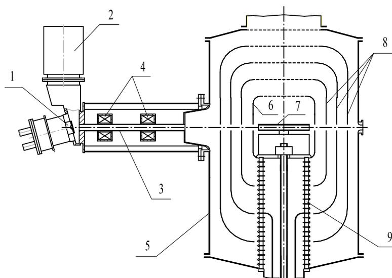
*Fig.1. Scheme of the powerful tandem accelerator: 1 – source of negative ions, 2 – vacuum pump, 3 – low energy beam line, 4 – magnetic lenses, 5 – vacuum tank, 6 – high-voltage electrode, 7 – charge exchange tube, 8 – intermediate electrodes, 9 – high-voltage insulator.*
