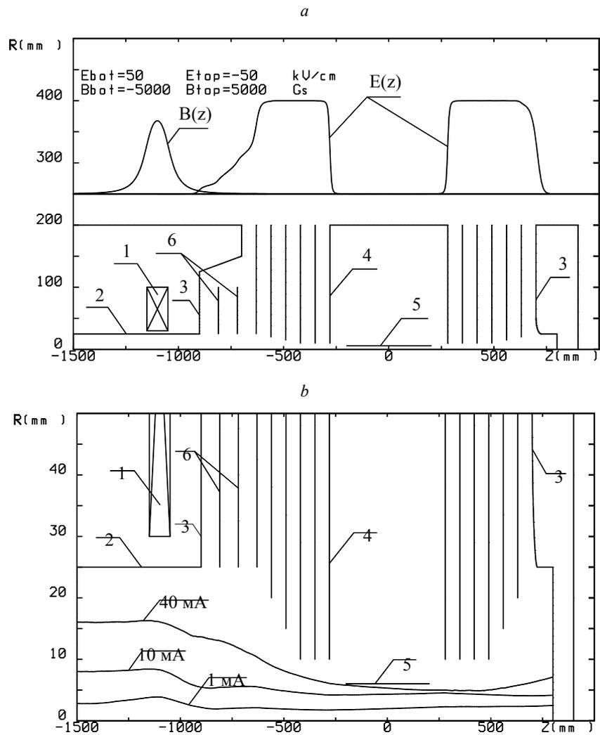
Fig. 6. Coordinated transport of 25 keV H beam through tandem accelerator according to “weak” focusing scheme: the ion-optical path geometry, calculated longitudinal distributions of the field (a) and the calculated envelopes of ion beams with current of 1 mA, 10 mA and 40 mA, spanning 95% of the current (b). The numbers mark: 1 – current coil, 2 – drift tube, 3 – vacuum tank, 4 – high-voltage electrode, 5 – charge-exchange tube, 6 – additional electrodes.
