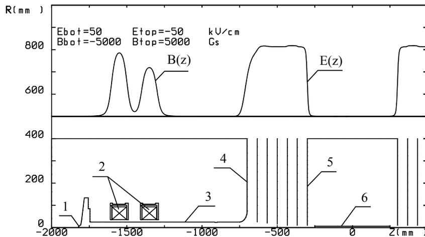
Fig. 12. Geometry of the ion-optical channel of tandem accelerator and calculated longitudinal distribution of the field for the scheme with “strong” focusing of  $H$  beam with current of 10 mA and initial energy of 25 keV. The numbers mark: 1- the ion source, 2 – magnetic lenses, 3 – drift tube, 4 – vacuum tank, 5 – high-voltage electrode, 6 – charge-exchange tube.
