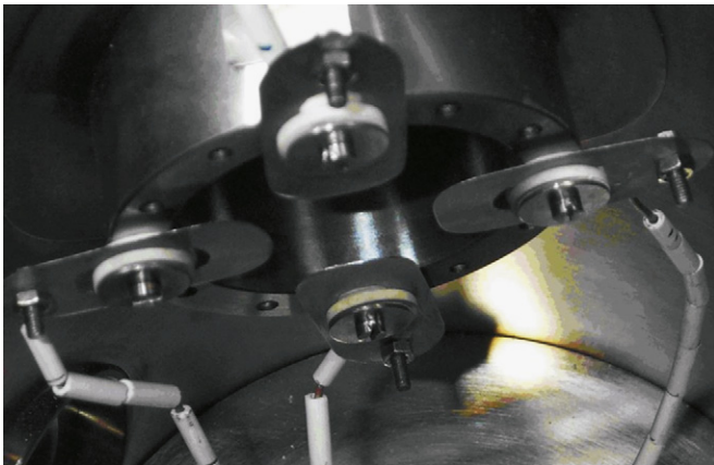
Fig. 2. Pick-up electrodes for control of proton beam intensity on high-energy tract periphery.
