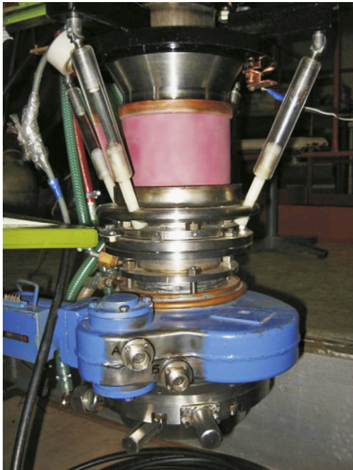
Fig. 6. Photo of the neutron producing target suspended on the ceramic insulator.
