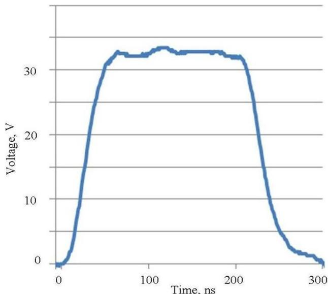
Fig. 2. Signal of the high voltage divider, proportional to the voltage on the exit unit (the amplitude of the pulse is 40kV).
