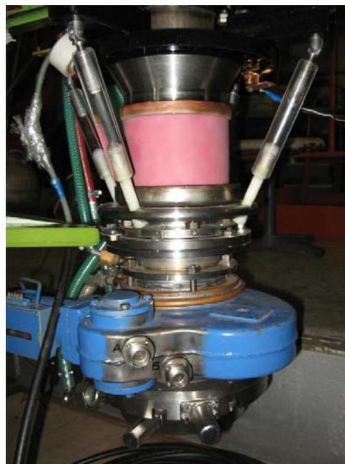
Fig. 3. The photo of the neutron producing target suspended on the ceramic insulator.
