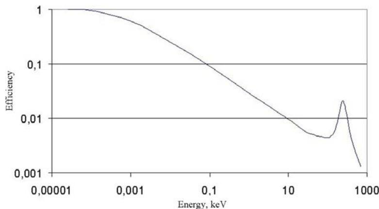
Fig. 4. Calculated detection efficiency as a function of neutron energy for the scintillator GS20.
