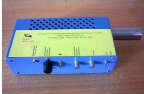
Fig. 6. The detector and power source assembled together with the accumulator.
