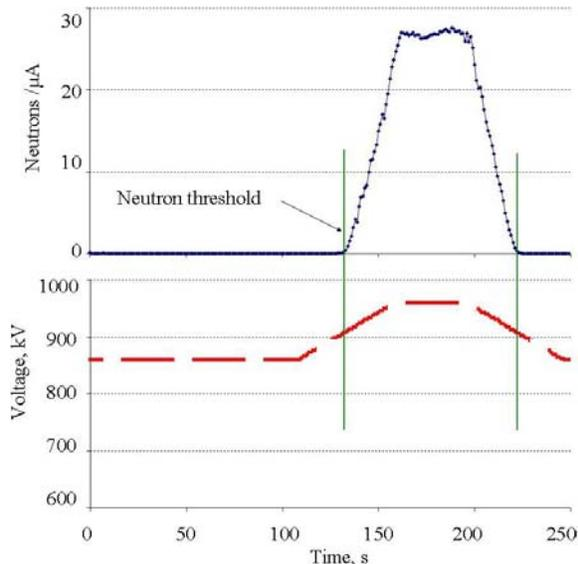
Fig. 7. The exact neutron production threshold. Interrupted line shows the voltage on a tandem depending on the time, solid line - the number of neutrons registered by the detector at this time and divided to the unit of proton beam current.
