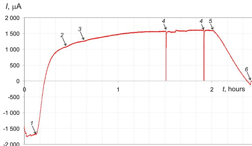
**Figure 4.** The time dependence of the ion beam current. Arrow 1 indicates the beginning of the gas flow in the stripper with a valve opening frequency of 1/10 Hz, 2 — 1/7 Hz, 3 — 1/5 Hz; arrow 4 marks the breakdown of the full voltage, 5 — turn off the gas supply, 6 — turn off power.
