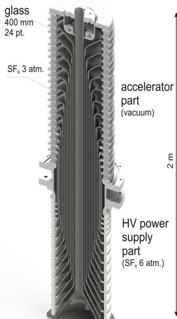
**Figure 2.** Scheme of the high-voltage feed-through insulator.
