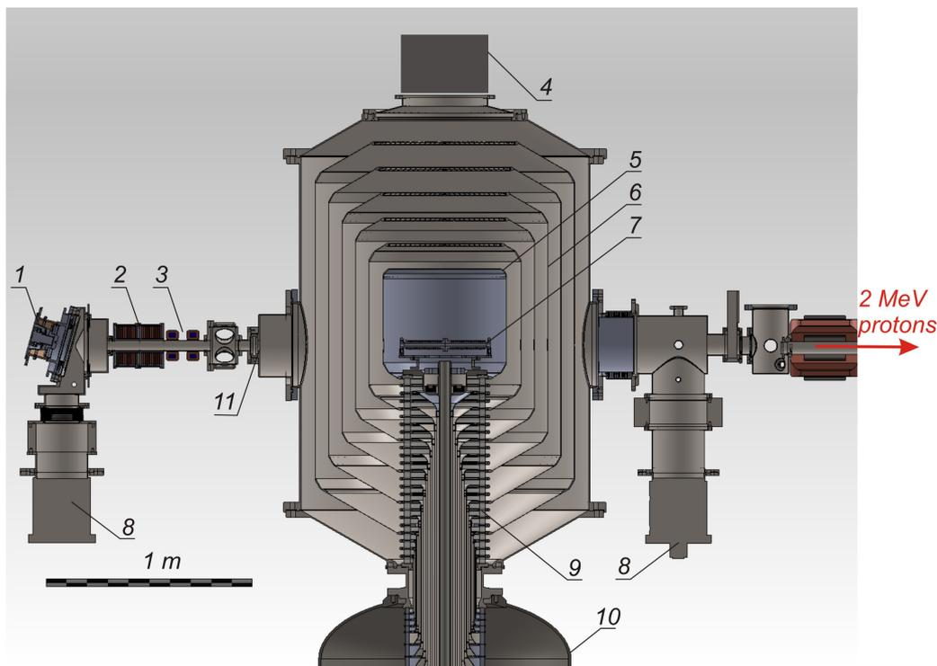
**Figure 1.** Tandem accelerator with vacuum insulation: 1 — source of negative hydrogen ions, 2 — magnetic lenses, 3 — correctors, 4 — cryogenic pump, 5 — high voltage electrode, 6 — intermediate electrodes, 7 — the gas stripper, 8 — turbomolecular pump, 9 — insulator, 10 — high-voltage power supply, 11 — inlet diaphragm.
