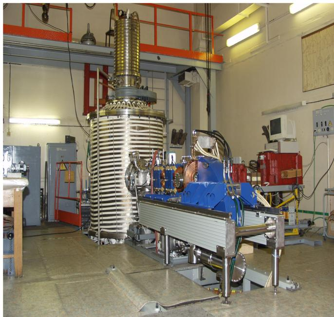
**Figure 3.** Photo of the tandem accelerator with vacuum insulation.
