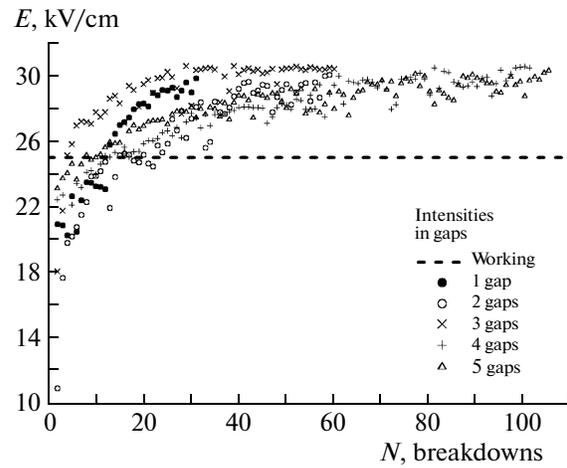
Fig. 5. Dependence of the intensity in the gaps on the number of breakdowns.
