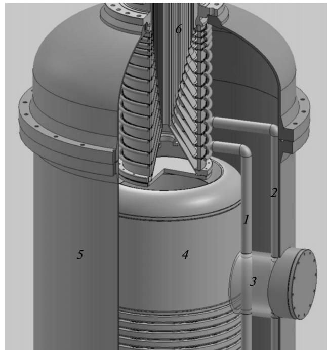
**Fig. 2.** Work tool for the single and serial connection of the gaps: (1) bar with a high potential; (2) earth bar; (3) insulator; (4) high-voltage electrode of the rectifier; (5) tank of the rectifier; and (6) gas part of the bushing insulator.
