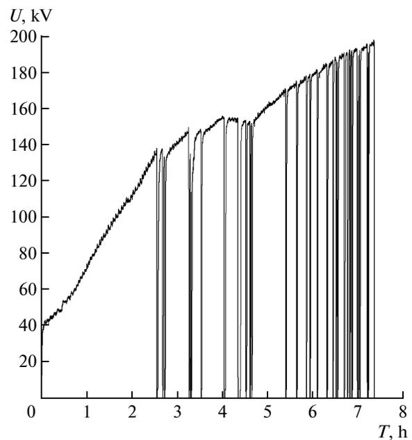
**Fig. 3.** Voltage buildup at the single gap.
