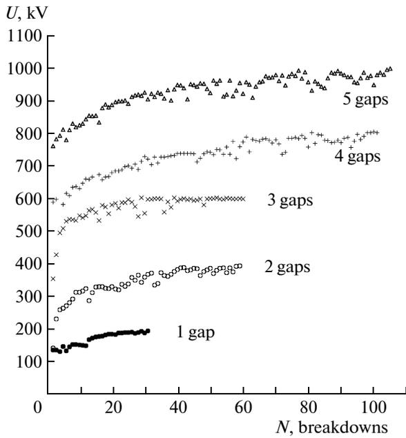
Fig. 4. Dependence of the breakdown voltage on the number of breakdowns.
