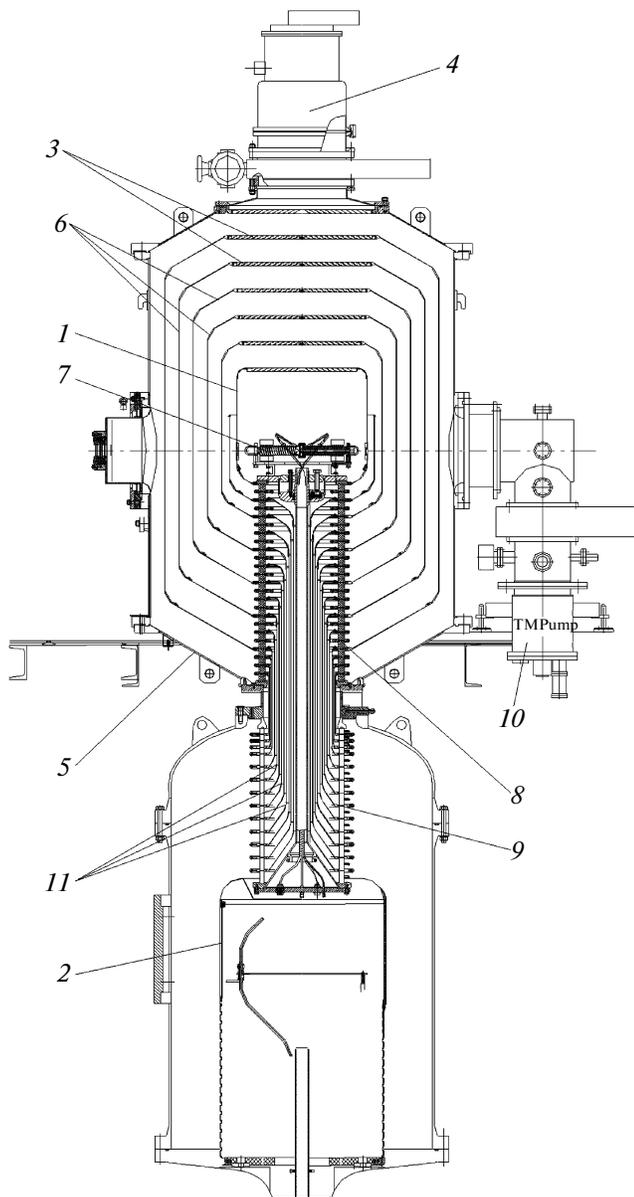
**Fig. 1.** General appearance of the six-gap tandem accelerator with the vacuum insulation: (1) high-voltage electrode of the tandem accelerator; (2) high-voltage electrode of the voltage source; (3) jalousie of the electrodes-screens; (4) cryogenic pump; (5) vacuum tank of the accelerator; (6) intermediate electrodes-screens; (7) gas stripping target; (8) vacuum part of the bushing insulator; (9) gas part of the bushing insulator; (10) turbo-molecular pump; and (11) internal coaxial cylinders.
