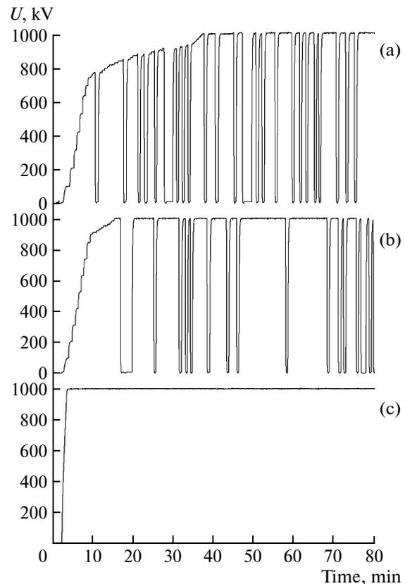
Fig. 6. Dynamics of reaching the operating voltage of the mode without breakdowns: (a) beginning, (b) middle, and (c) end of aging.
