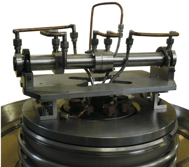
Fig. 2. Photo of the stripping target placed on the feedthrough insulator.
