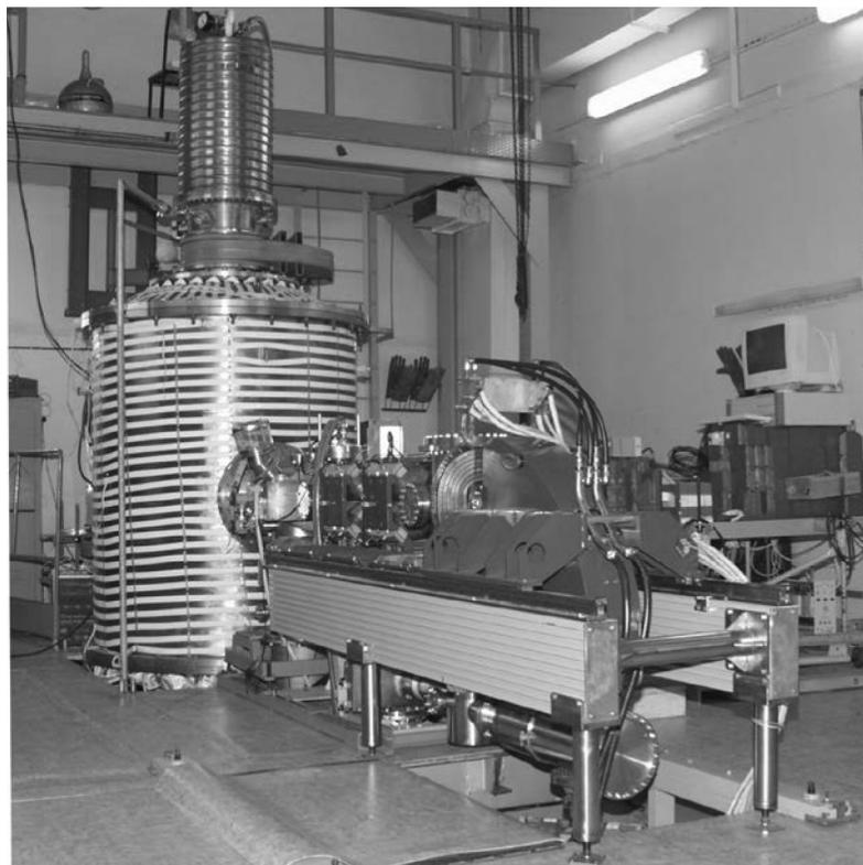
**Fig. 6.** Photo of a tandem accelerator with vacuum insulation.
