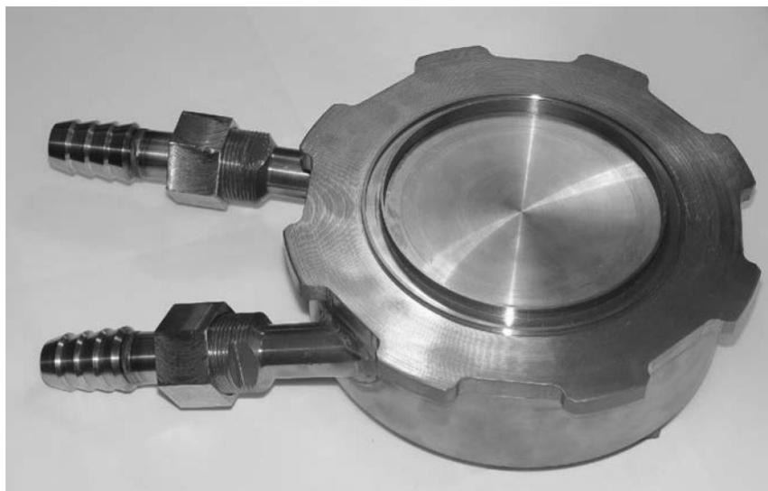
Fig. 19. Photo of the target unit and beam receiver.
