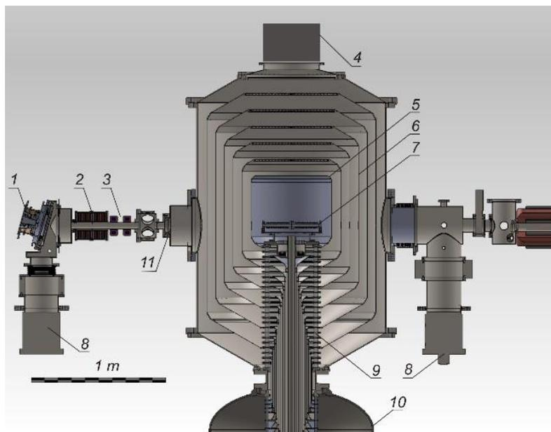
**Figure.3** Tandem accelerator with vacuum insulation: 1 – source of negative hydrogen ions, 2 – magnetic lenses, 3 – correctors, 4 – cryogenic pump, 5 – high voltage electrode, 6 – intermediate electrodes, 7 – gas stripping cell, 8 – turbomolecular pump, 9 – insulator, 10 – high-voltage power supply, 11 – inlet diaphragm.
