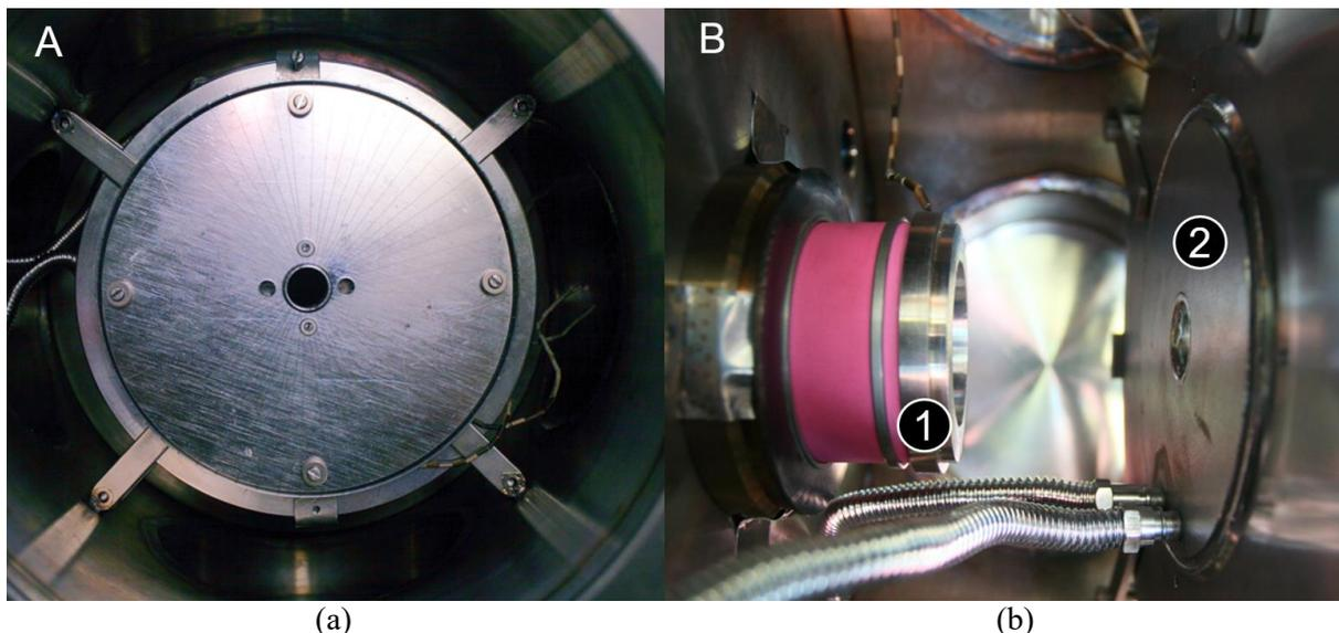
**Figure.6.** (a) Argon detector with grid under voltage. (b) 1 – Metal circle under voltage, 2 – Water-cooled diaphragm.
