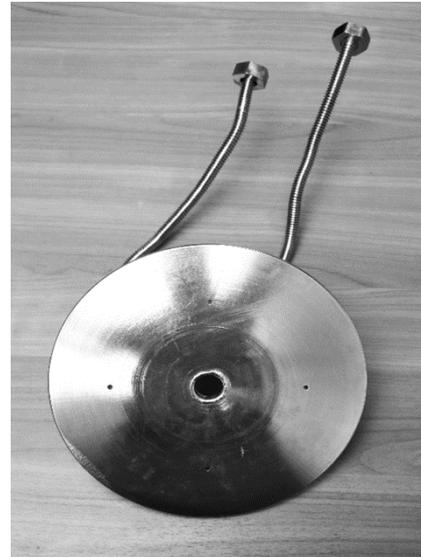
**Figure.5** Water cooled diaphragm
