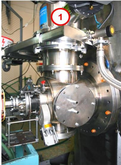
**Figure.4** Input node. 1– Cryopump
