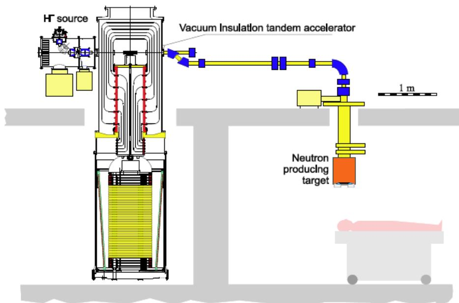
**Figure. 2** Accelerator based on neutron source for BNCT
