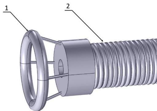
**Figure.10** 1– Electrostatic ring. 2–Stripping target
