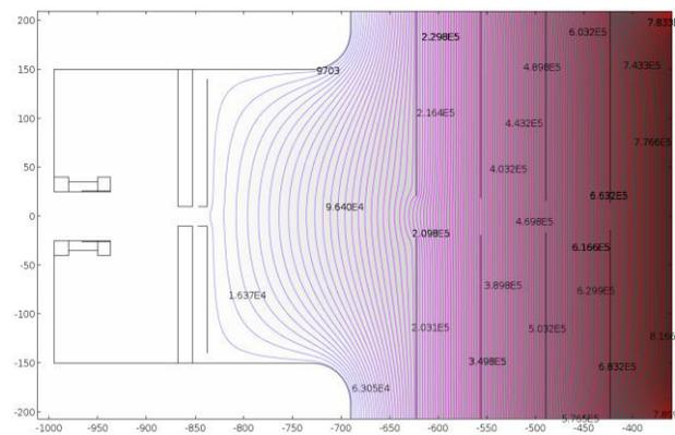
Figure 2: Calculated field distribution inside the vacuum chamber at the entrance to the accelerator.
