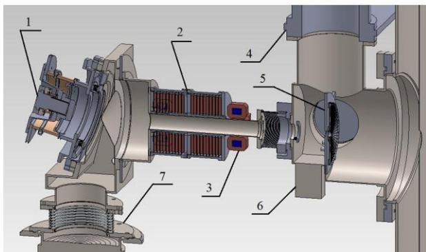
Figure 1: Low-energy part of accelerator. 1 – H<sup>-</sup> ion source, 2 – magnetic lenses, 3 – corrector, 4 – cryosorption pump, 5 – cooled diaphragm, 6 – D-Pace wire scanner, 7 – differential pumping system.
