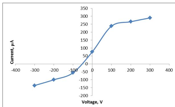
Figure 5: Volt-ampere characteristics of the wire scanner.
