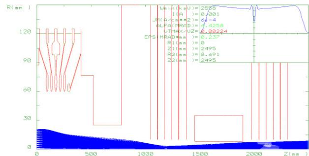
Figure 4. Transportation of 1 mA beam through the pre-accelerator tube and the VITA.
