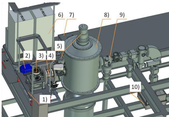
Figure 3. Facility arrangement with the beam injector equipment: 1 – Faraday cage with the injector, 2 – for-pump, 3 – H<sup>-</sup> ion source, 4 – pre-acceleration tube, 5 – cryo pumps, 6 – Faraday cage with the injector power and control cabinets, 7 – isolating transformer, 8 – vacuum
