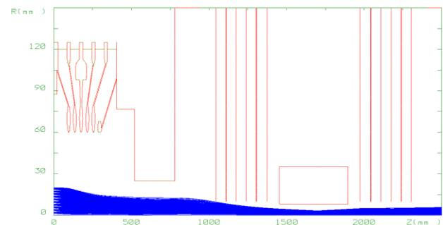
Figure 5. Transportation of 10 mA beam through the pre-accelerator tube and the VITA.
