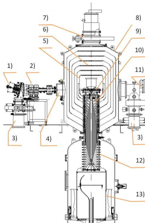
Figure 1. Scheme of the VITA facility: 1 – H<sup>-</sup> ion source; 2 – low energy beam line; 3 – turbomolecular pump; 4 – entrance volume of the accelerator; 5 – high voltage electrode; 6 – electrode shutters; 7 – cryo pump; 8 – accelerator vacuum volume; 9 – stripping target; 10 – feedthrough insulator (vacuum part); 11 – high energy beam line; 12 – feedthrough insulator (gas part); 13 – high voltage source.
