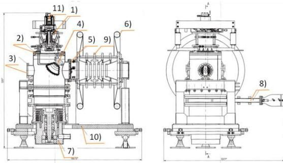
Figure 2. New injector design: 1 – 15 mA H<sup>-</sup> ion source; 2 – positioning flange; 3 – vacuum chamber; 4 – beam magnet; 5 – diaphragm with the beam diagnostics; 6 – high voltage screen; 7 – turbomolecular pump; 8 – vacuum valve; 9 – pre-acceleration tube; 10 – insulated support; 11 – Cs heater.
