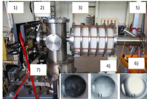
Figure 7. Stand for preliminary accelerator tube testing: 1 – 15 mA H<sup>-</sup> ion source; 2 -vacuum chamber; 3 – accelerator tube; 4 – Faraday cup; 5 – view port; 6 – location of the tantalum foil; 7 – vacuum valve and pumping. Photo of the tantalum target: a) no beam; b) 6 mA, no acceleration; c) 6 mA @ 50.5 kV acceleration (82 keV total energy).
