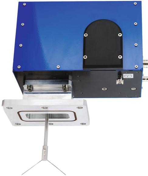
Fig. 3. A photo of the OWS-30 wire scanner.
