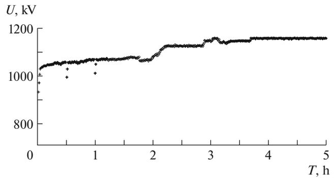
**Fig. 15.** A graph of the voltage  $U$  at the accelerator versus time  $T$  when the voltage is increased and maintained at a level of 1.15 MV.
