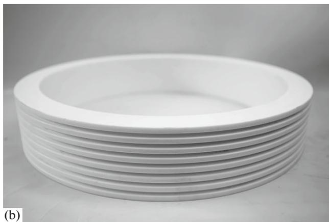
**Fig. 5.** The ceramic insulators with (a) smooth and (b) ribbed outer surfaces.
