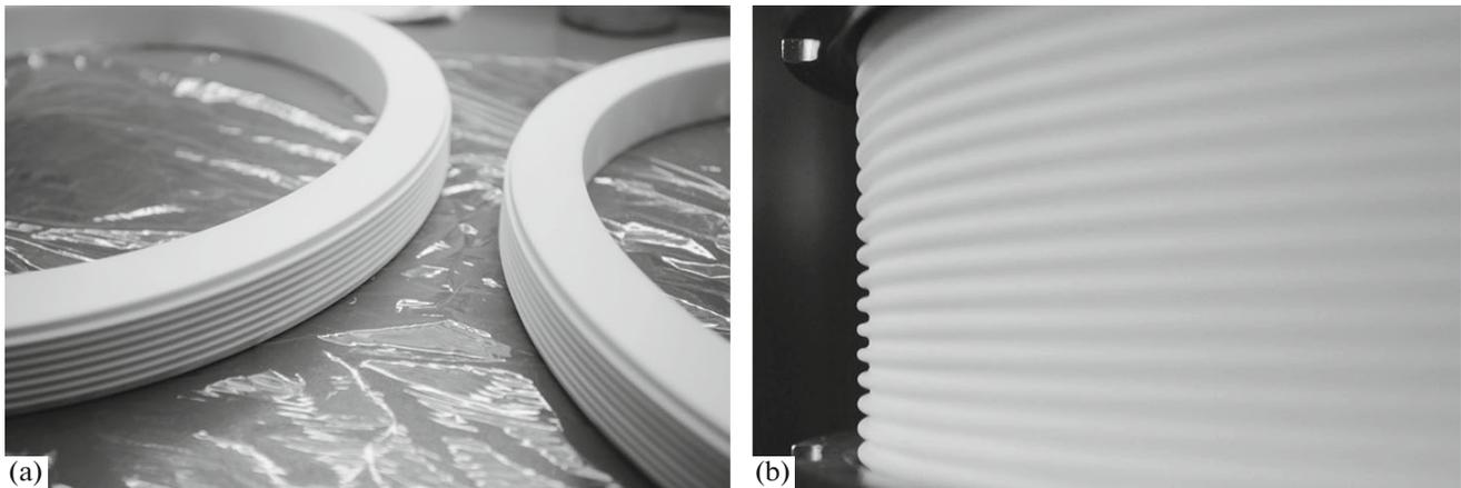
**Fig. 12.** The ceramic insulators with a ribbed outer surface and a height of (a) 35 and (b) 70 mm.
