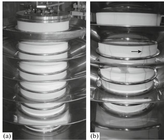
**Fig. 11.** Photos of the smooth ceramic surface of the insulator (a) before and (b) after the training with traces of breakdowns. The arrow points to one of the tracks formed after the breakdown.
