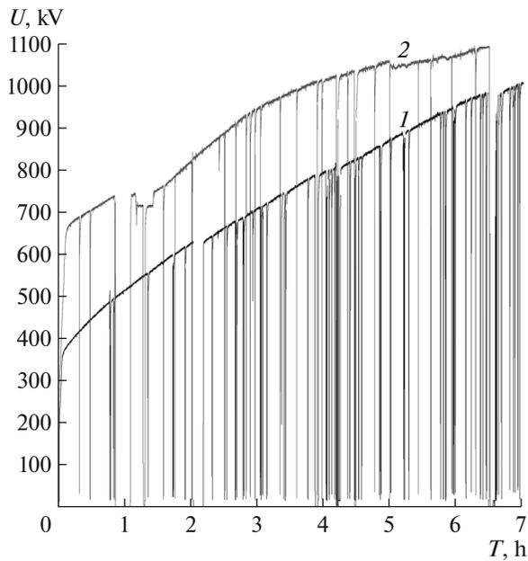
**Fig. 13.** Graphs of the first voltage rise at the accelerator: (1) for the smooth ceramic surface of the insulator and (2) for the ribbed ceramic surface.
