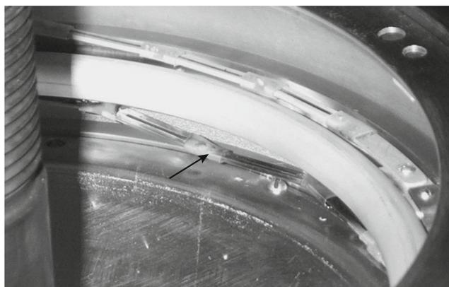
**Fig. 4.** The sagging and burnout of a part of the voltage divider (shown by the arrow) inside the feedthrough insulator.
