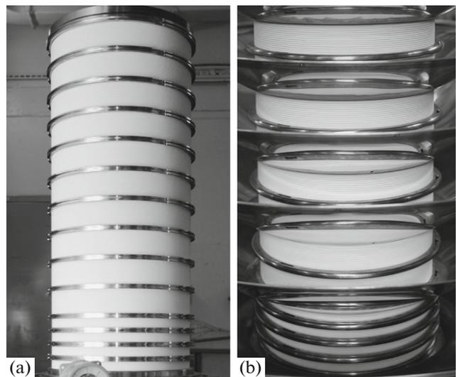
**Fig. 16.** Photos of the ribbed ceramic insulator surface (a) before and (b) after the training.
