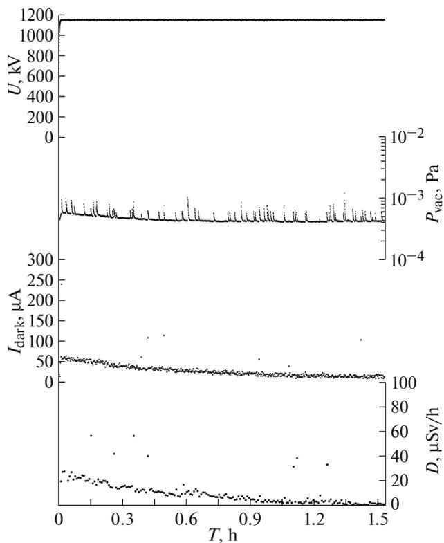
**Fig. 9.** Graphs of the voltage  $U$ , residual pressure  $P_{vac}$ , dark current  $I_{dark}$ , and the bremsstrahlung dose rate  $D$  of the accelerator when the voltage is maintained at a level of 1.15 MV.
