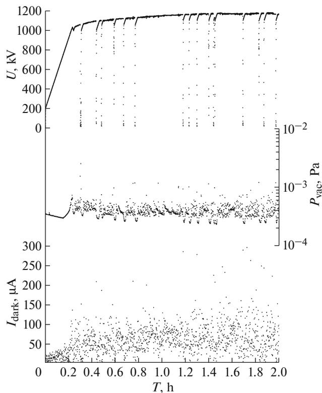
**Fig. 8.** Graphs of the voltage  $U$ , residual pressure  $P_{vac}$ , dark current  $I_{dark}$  at the accelerator vs. time  $T$  during the voltage rise.
