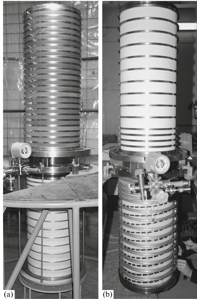
**Fig. 7.** Photos of the feedthrough insulator with (a) 35-mm-high glass rings and (b) with 73- and 35-mm-high smooth ceramic rings.
