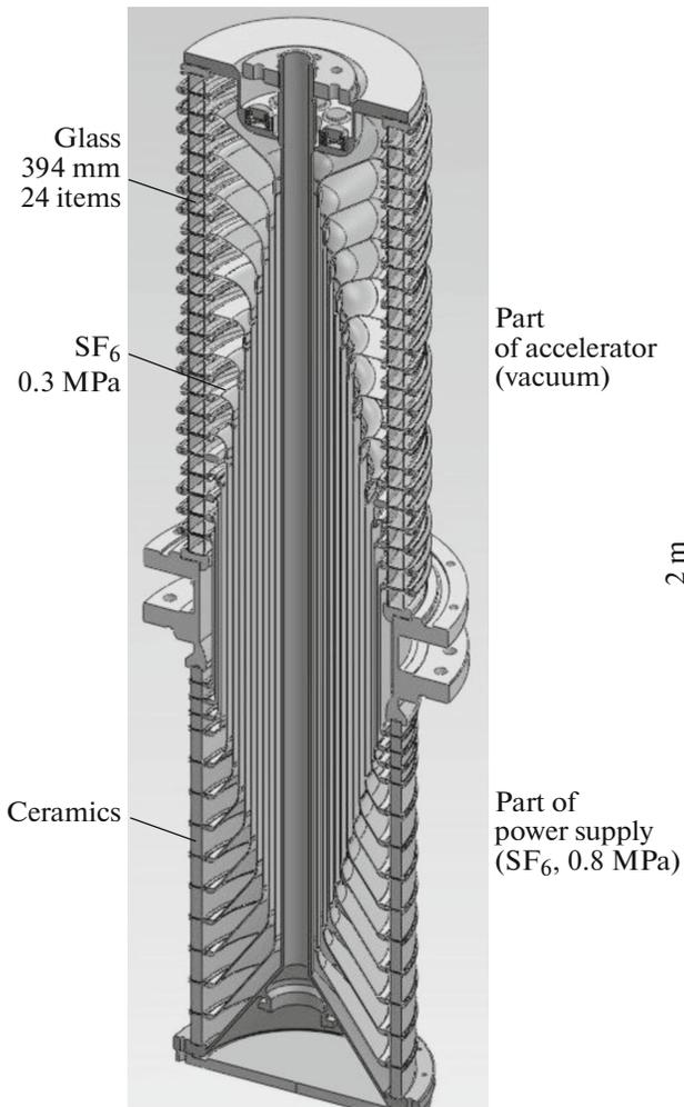
**Fig. 2.** A diagram of the feedthrough insulator of the accelerator.
