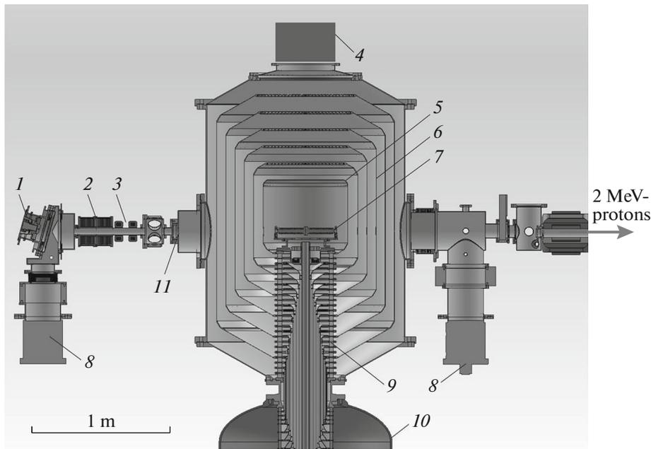
**Fig. 1.** The vacuum-insulated tandem accelerator: (1) source of negative hydrogen ions, (2) magnetic lenses, (3) correctors, (4) cryogenic pump, (5) high-voltage electrode, (6) intermediate electrodes, (7) gas stripping target, (8) turbomolecular pump, (9) feedthrough insulator, (10) high-voltage power supply, and (11) the location of the entrance diaphragm of the accelerator.
