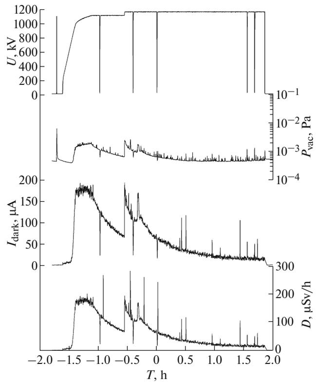
**Fig. 3.** Graphs of the accelerator-voltage rise.
