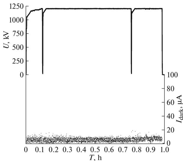
**Fig. 14.** Graphs of the voltage  $U$  and dark current  $I_{\text{dark}}$  at the accelerator vs. time  $T$ .
