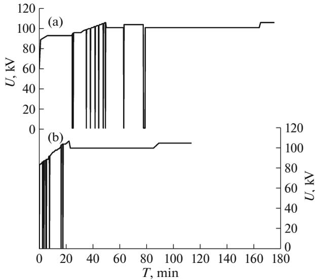
**Fig. 6.** The voltage rise at the 73-mm-high insulators with (a) smooth and (b) ribbed outer surfaces.
