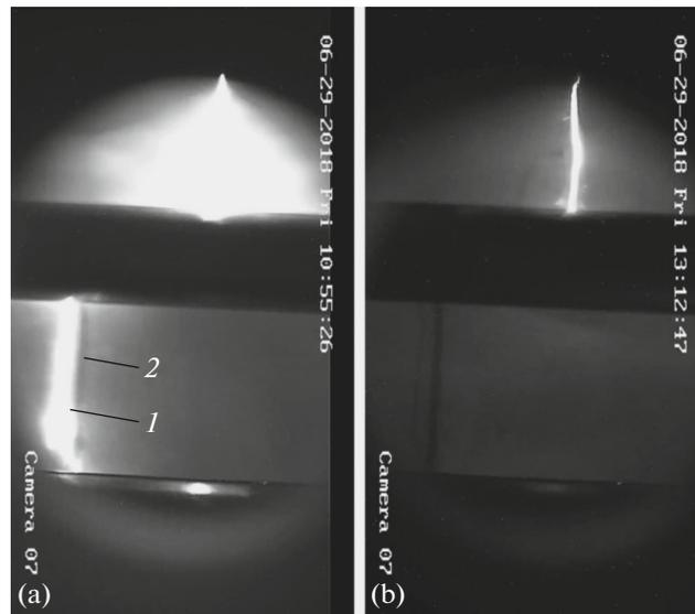
**Fig. 10.** Photos of breakdowns over the insulator surface: (1) current breakdown and (2) track formed from a previous breakdown.
