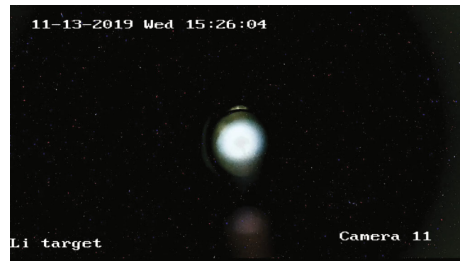
Fig. 4. The luminescence recorded by a Hikvision video camera when a lithium target is irradiated with a proton beam.
