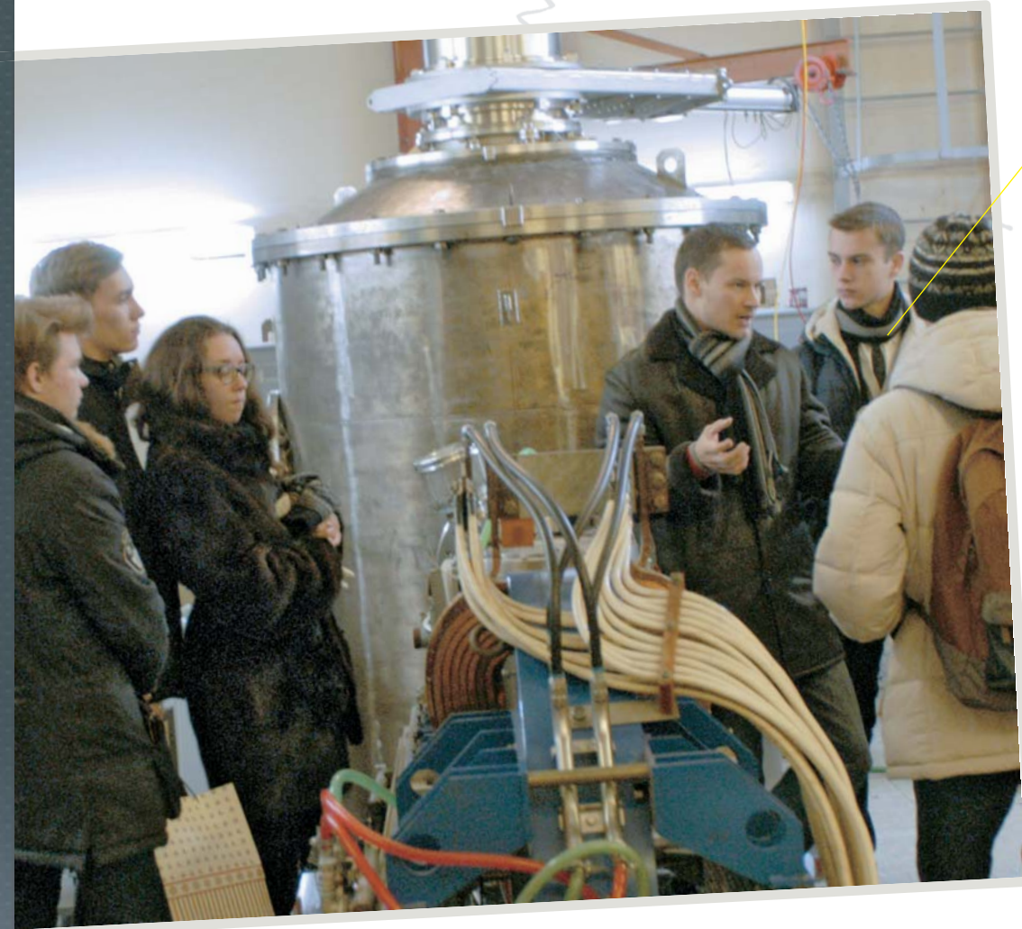
The core part of the BNCT facility is a new-type accelerator generating a beam of epithermal protons. Photo: Alexander Makarov, researcher at the BNCT laboratory, explains the working principles of the unique accelerator to a group of secondary school students from Novosibirsk
