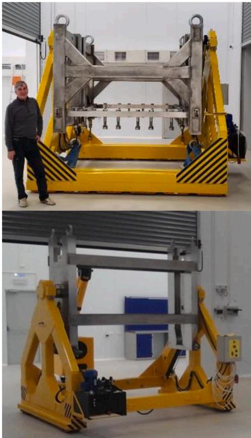
**Fig. 14.** Clean room in the BINP with port plug handler inside (top) and DSM equatorial port handler installed (bottom).
