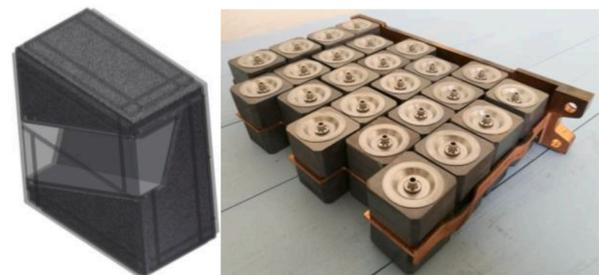
Fig. 3. Drawing of the previous design steel box with boron carbide powder for DSM Equatorial Port Plug #11 with cutouts for diagnostics (left) and a photo of the prototype tray in its current design (right). For better thermal conductivity, the tray in the prototype was made of bronze; however, calculations showed that bronze would not withstand expected loads, and for that reason it was decided to use steel 316L(N)-IG instead.
