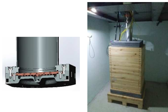
Fig. 3. Model of the lithium target assembly (left) and photo of the concentrator (right).
