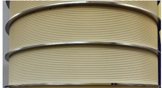
Fig.3. Corrugated surface upper vacuum part of the individual insulator.
