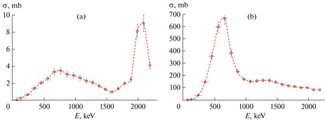
Fig. 8. Measured cross-section of the reactions  $^{11}\text{B}(p,\alpha_1)^8\text{Be}$  (a) and  $^{11}\text{B}(p,\alpha_1)^8\text{Be}^*$  (b).
