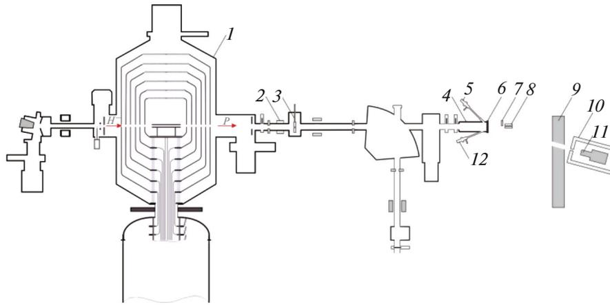
**Fig. 1.** Schematic diagram of the experimental setup: (1) tandem accelerator with vacuum insulation, (2) noncontact current sensor, (3) retractable cooled collimator, (4) target unit, (5 and 12)  $\alpha$ -spectrometer, (6) lithium target, (7) temporarily placed lead sheet, (8) fast neutron spectrometric radiometers with a diamond detector, (9) temporarily constructed concrete wall, (10) lead collimator, (11)  $\gamma$ -spectrometer.
