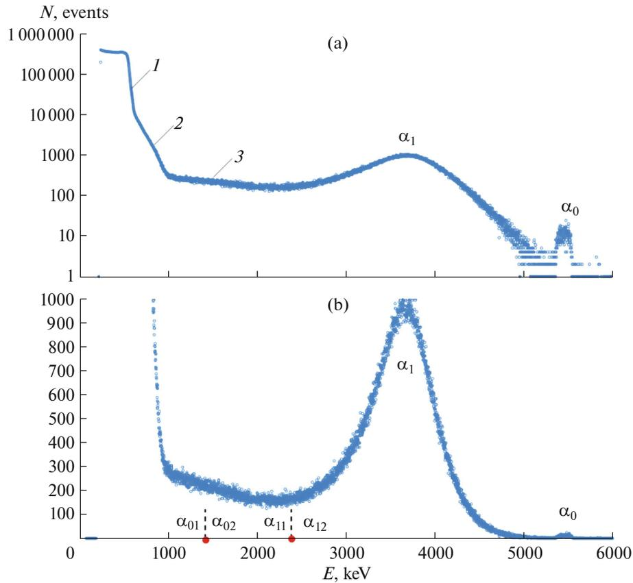
**Fig. 7.** Signal of the  $\alpha$ -spectrometer used in a 0.6-MeV deuteron beam and an angle of  $168^\circ$ : (1–2) backscattered deuterons ((1) single events, (2) double), (3)  $\alpha$ -particles.
