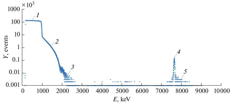
**Fig. 3.** Spectrum of charged particles registered by the  $\alpha$  spectrometer at a proton energy of 1 MeV: (1–3) backscattered protons (1) single events, (2) double, (3) triple, (4)  $\alpha$  particles, (5) simultaneous detection of  $\alpha$  particle and proton.
