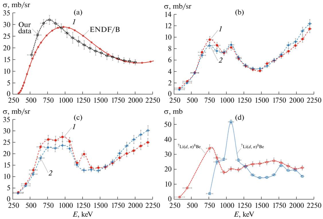
**Fig. 6.** Measured cross section of the reaction  ${}^6\text{Li}(d, \alpha){}^4\text{He}$  (a),  ${}^7\text{Li}(d, \alpha){}^5\text{He}$  (b),  ${}^7\text{Li}(d, n\alpha){}^4\text{He}$  (c),  ${}^7\text{Li}(d, n){}^8\text{Be}$ , and  ${}^7\text{Li}(d, n){}^8\text{Be}^*$  (d); (I) at an angle of  $135^\circ$ , (2) at an angle of  $168^\circ$ .
