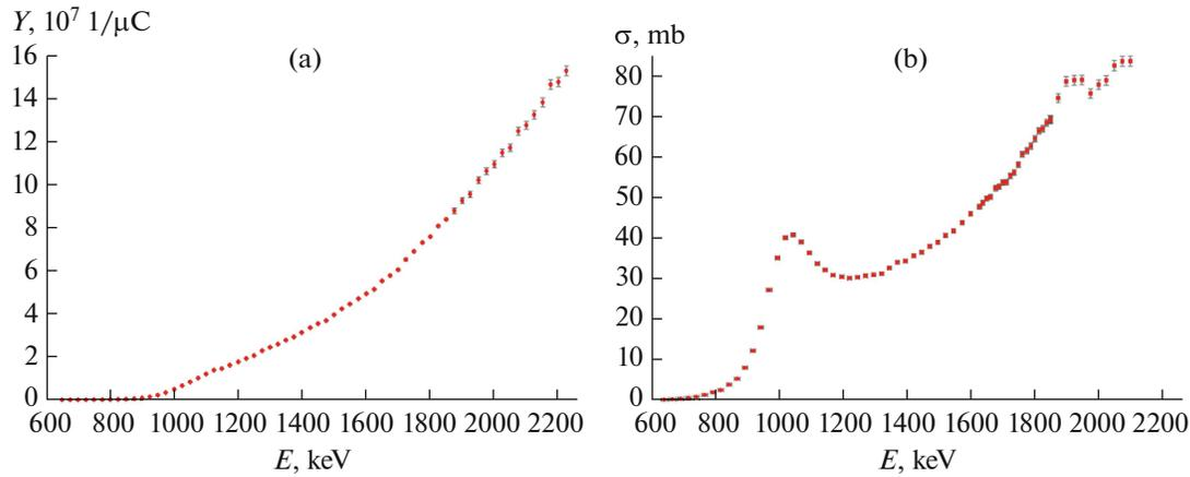
**Fig. 2.** The yield of 478-keV photons from a thick lithium target with natural content of lithium isotopes (a) and the cross sections of the reaction  ${}^7\text{Li}(p,p'\gamma){}^7\text{Li}$  as a function of the proton energy  $E$  (b).
