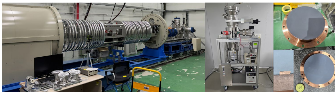
Fig. 1. Tandem accelerator(left), Lithium evaporation system(middle) and Lithium target(right)
