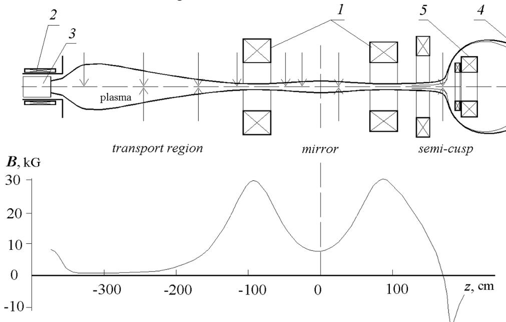
Fig. 1. Scheme of AMBAL-M experiments. 1— mirror coils, 2 — gun solenoid, 3 — plasma gun, 4 — plasma receiver, 5 — semi-cusp coil. The arrows of the cross sections where Langmuir probes were measured, from below — magnetic probes.
